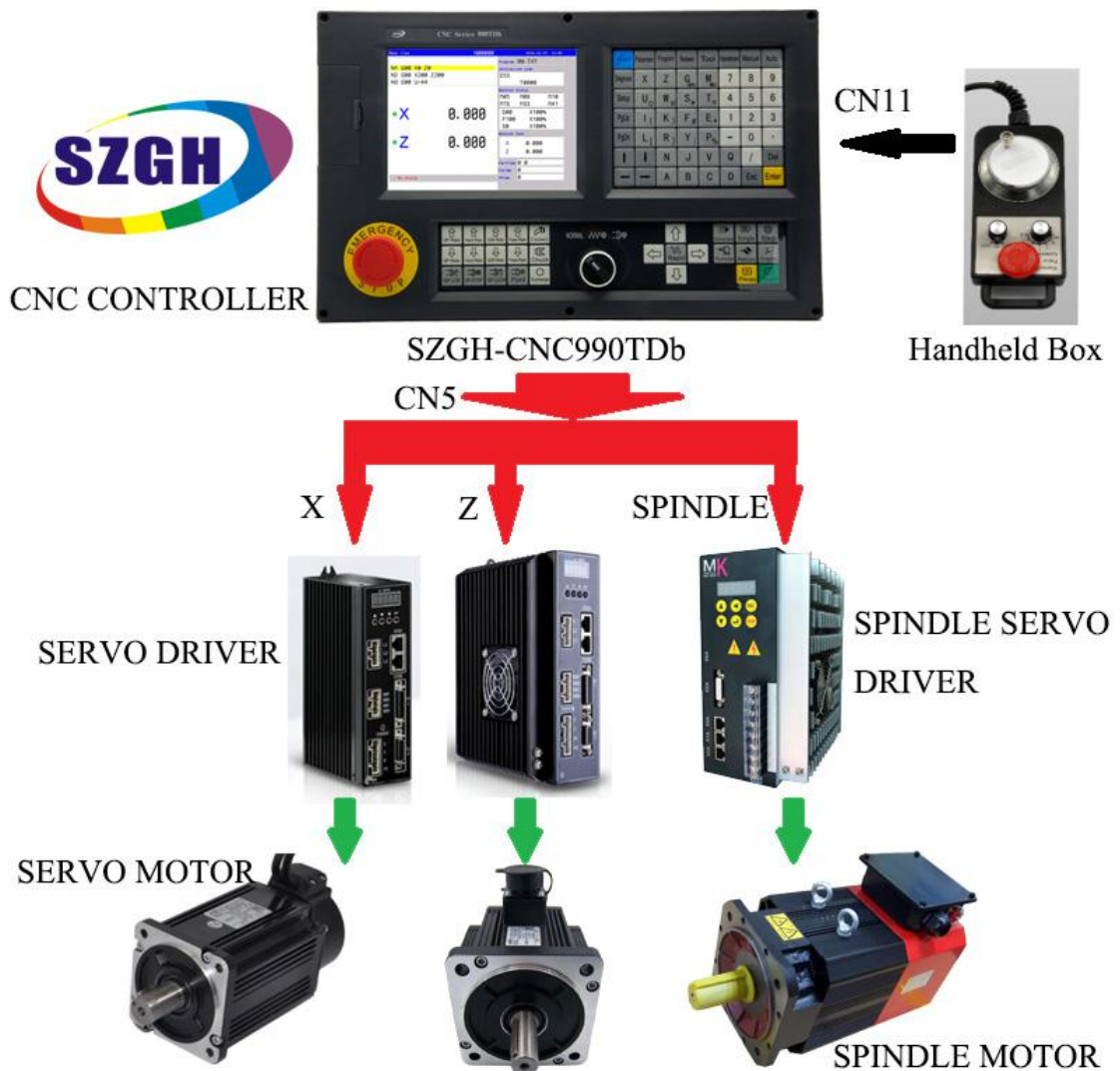
Fig1.2 Wiring Sketch for Total CNC Lathe System
