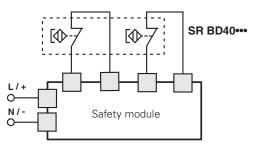
Connection with safety modules CS AR-05 or CS AR-06
