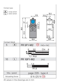
The FR 5F1-M2, FR 10F1-M2 switches are applied on electrical panel doors and are used when opening the door to turn on any signalling devices (e.g. three-phase flashing, etc.). Maintenance personnel of the panel can simulate the closing of the door by pressing the blue button. When maintenance is performed by simply closing the switching cabinet door, the switch functionality will be automatically reset.
