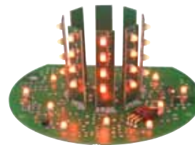
48 LEDs – light emission in all directions
